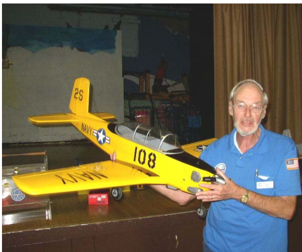
Harvey's Hanger 9 T34 Mentor uses a .40 motor and weighs 7lb 3oz. The ruder was modified to move freely. Harvey claims that the grimace on his face reflects what this plane has put him through. Good looking results, Harv! ...The AIRPLANE, that is!
