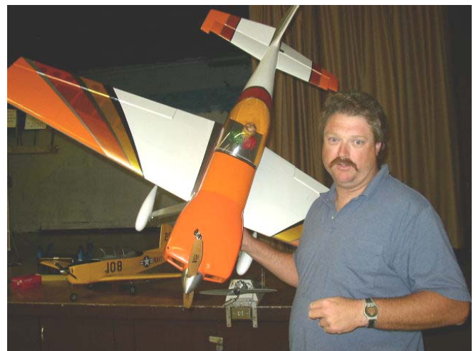
After Jeff lost an aileron on this Sig Cap 231 it took him six months to rebuild. A pumped Saito 180 swings an 18x6 prop.
