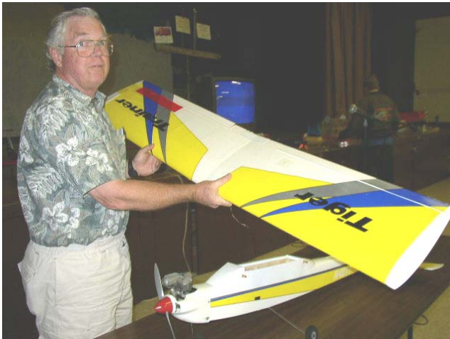
George's Tiger Trainer is stock except for some tape on the control surfaces and smaller servos. A Magnum .46 spins a 10x6 prop at 14,500 rpm. The trainer race max rpm is 13,500. An ARF trainer is a cheap and simple way to get into racing. George gathers many points despite the Tiger's "suarish" wheels.
