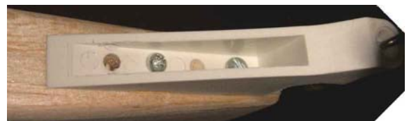
The plywood triangle doubles the fuselage bottom just enough to accept a nice tail wheel bracket like this one.
