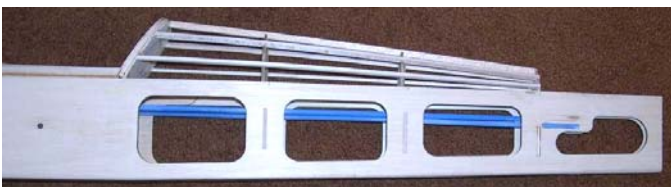
The Sullivan #505 Pushrods shown here perform much better than the generic plastic tubes included with the kit.
